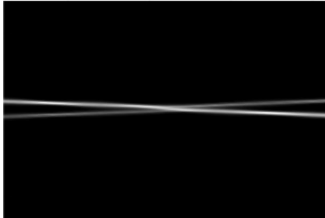
Figure 7. Two crossing self-induced waveguides with intensity ratio 2.
