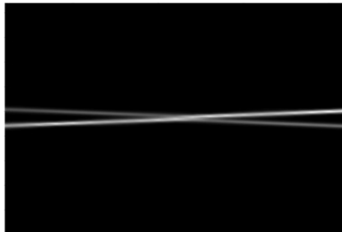
Figure 3. Two crossing self-induced waveguides with intensity ratio 0.5.
