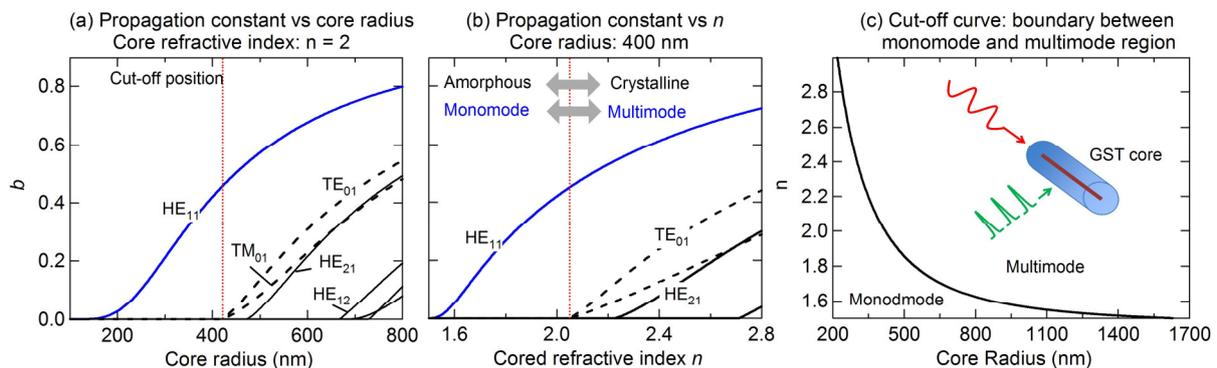
**Fig. 1** Normalized propagation constant as a function of core radius when core refractive index is fixed to 2 (a) and as a function of core refractive index when core radius is fixed to 400 nm (b) for a few low-order fiber modes. (c) Cut-off curve defines boundary between monomode and multimode region.
