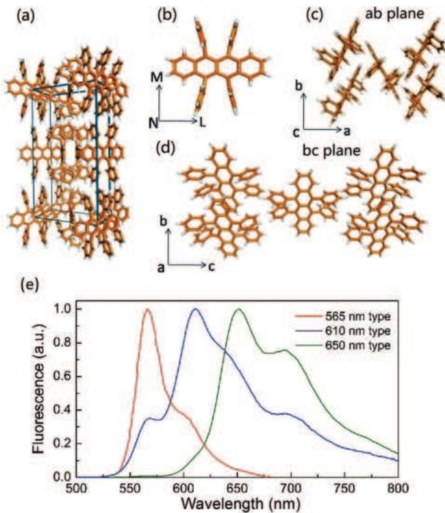
FIG. 1. (Color online) (a) Rubrene crystal structure. (b) Rubrene molecular structure. (c) Molecular packing on *ab* facet. (d) Molecular packing on *bc* facet. (e) Three types of steady-state fluorescence spectra in rubrene crystals.
