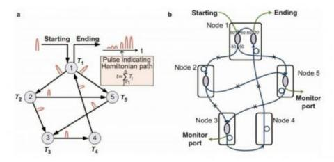
(a) The optical oracle's approach to solve the Hamiltonian path problem on a network with five nodes. An optical pulse is injected into the optical network and travels along all possible paths. A Hamiltonian path exists if a pulse returning to node 1 is observed after a delay equal to the total delay of the entire network. (b) Actual design of the optical oracle with optical fiber components. Credit: Wu, et al. ©2014 Nature
