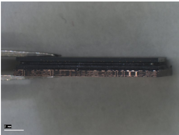
Figure : Application processor with RAM stacked above
